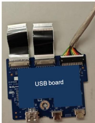
**S12** Assemble “USB board” to “Middle Frame” and fix it by screw\*1
