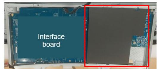
**S22** Unlock 10 PCBA screws to disassemble “Interface board”, “Power board” and “LED Driver board” from “Main Shielding”
