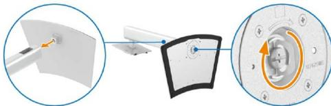
**S23** Attach the stand assembly to the monitor
