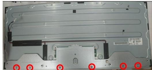
**S21** Disassemble "MYLAR Power" from "Main Shielding"
