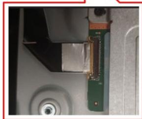
**S8** Adhere a yellow tape to fix "FFC EDP" connector
