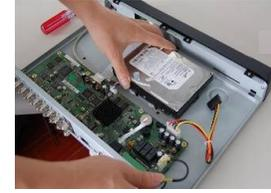
3. Fix the HDD firmly.
