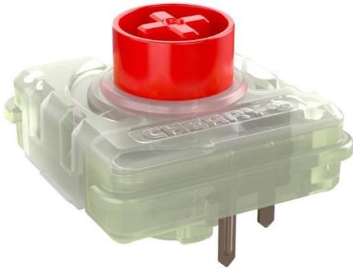
**Cherry MX Low Profile RGB Switches** with reduced 3.2mm travel distance and 1.2mm actuation point. Rated for 50 million+ lifespan to never let you down.
