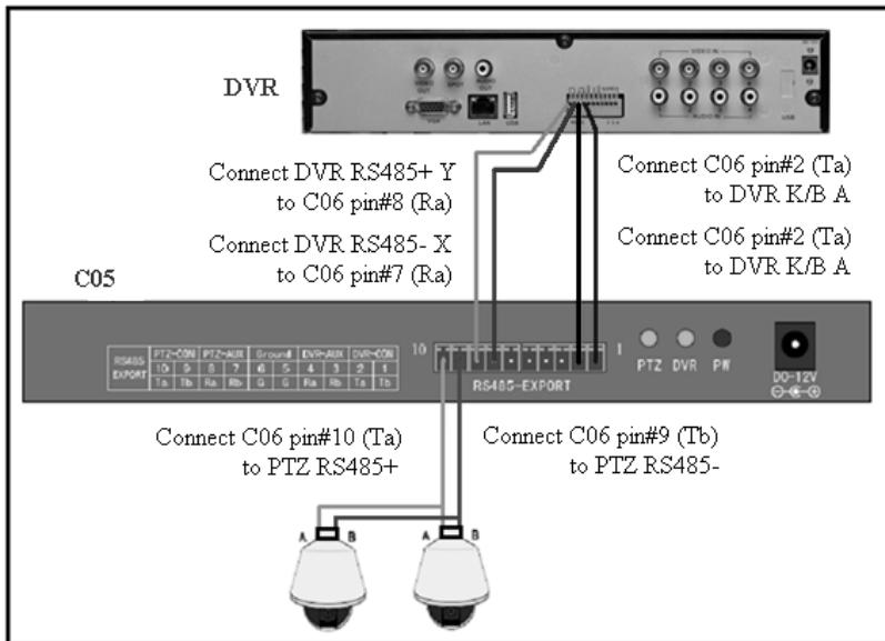
You can connect up to 32 DVRs, up to 15 C06 keyboards and up to 256 PTZ cameras on the same area (physical connection) where the RS485 cables do not extend over 1200 meters.
