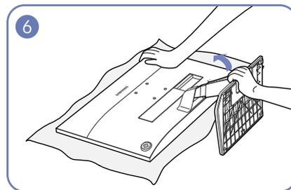
Hold the main body of the product with your hand, as shown in the figure. Hold and rotate the assembled stand until it fits exactly into the stop position.
