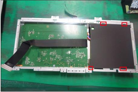
Use a Philips-head screwdriver to remove 7pcs screws for interface board and power board. Turn over the bracket and disconnect the camera cable.
