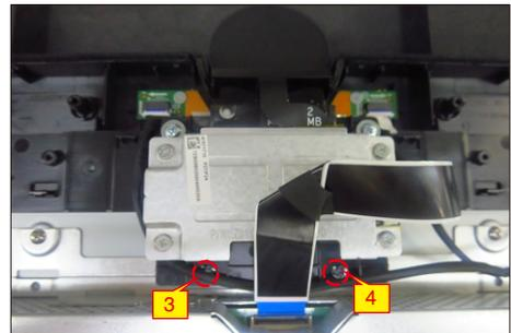
Use a Philips-head screwdriver to remove 4pcs screws for unlocking the bracket chassis with the panel, then disconnect the touch cable away from the connector of the main board.
