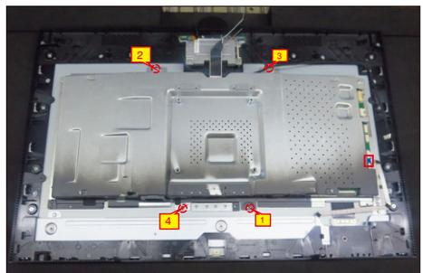
Disconnect the LVDS cable away from the connector of the panel module, then lift up and take away the bracket chassis and put it on a protective cushion.
