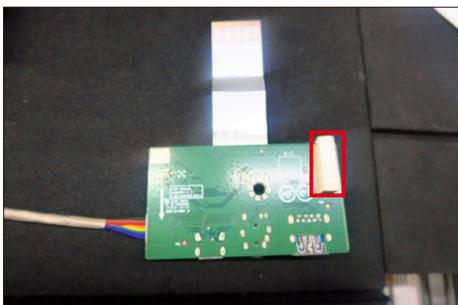
Locate the USB board into the hook of the middle frame. Use a Philips-head screwdriver to tighten 1pcs screw for locking the USB unit with the middle frame, then connect the two USB cables and Mic cable to the connectors of main board.
