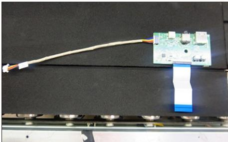
Tearing off 2pcs aluminum foil for releasing the connector and cable. Use a Philips-head screwdriver to remove 6pcs screws for unlocking the speakers with middle frame.
