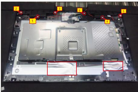
Disconnect the speaker cable away from the board, then release the speakers from the probers of the middle frame. Disconnect the panel lamp cable away from the connectors of the main board and panel.
