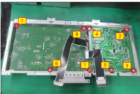
S21 Remove the power board and interface board from the bracket chassis module carefully, and then disconnect all of the cables.
