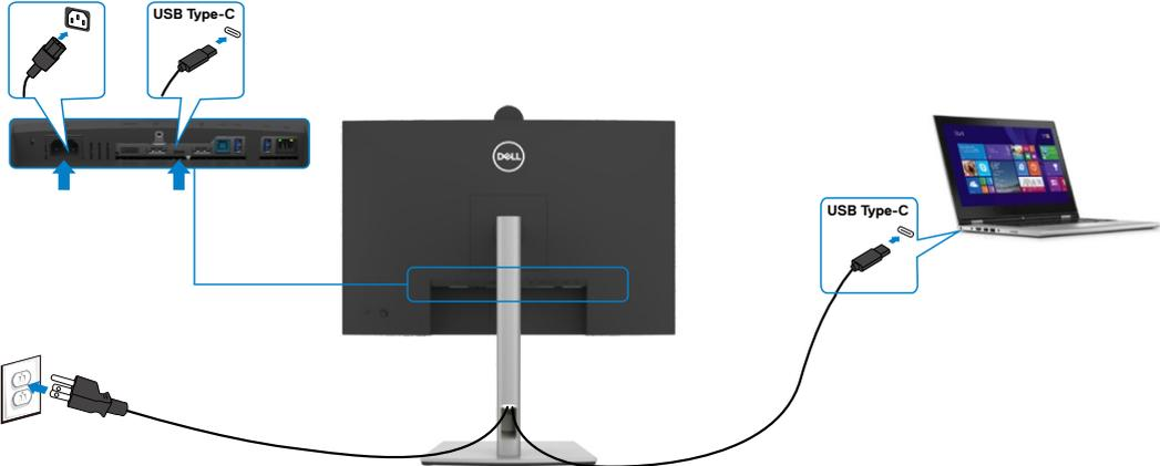
Connecting the monitor for USB-C Multi-Stream Transport (MST) function
