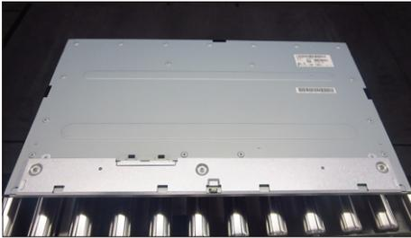
S19 Remove the Mylar tape from the hooks of the bracket chassis.
