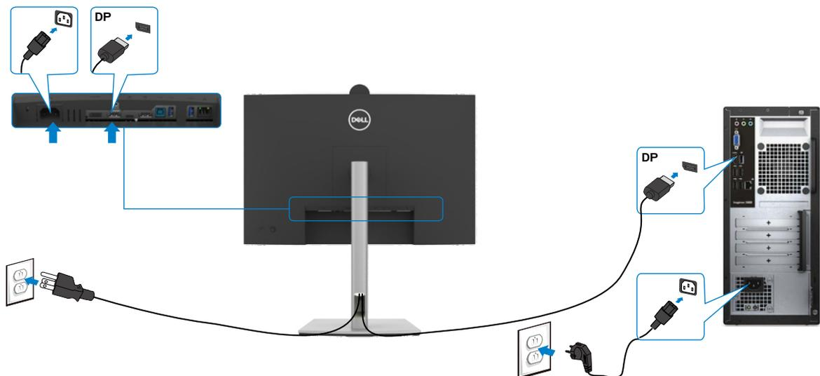
4. How to connect and disconnect power cable/ connectivity cable
