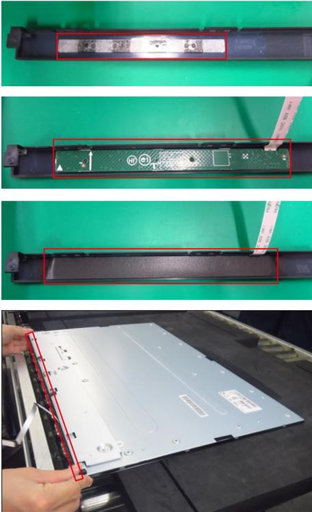
**S7** Take 1pcs left Mic board, 1pcs right Mic board and some essential cables, then assemble 1pcs rubber with left Mic board and assemble 1pcs rubber with right Mic board, then connect left Mic board right Mic board with cables as the picture below shown.
