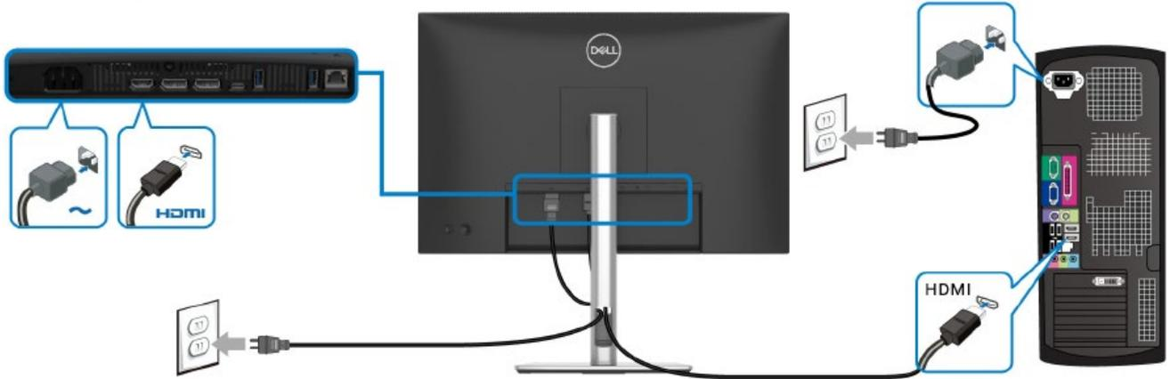
**Connecting/ disconnecting the monitor for RJ45 cable (optional) and Power cable**
