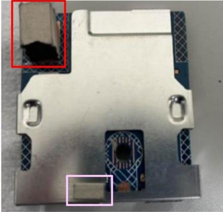
**S11** Disassemble “USB board” from “USB Shielding”
