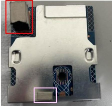
**S14** Assemble “USB board” with “Middle Frame”
