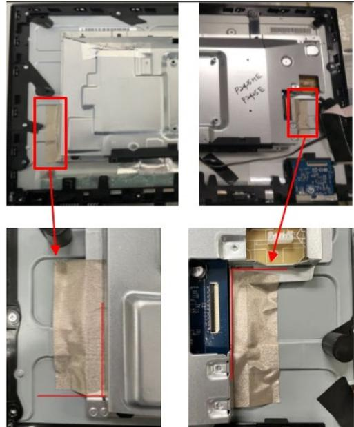
**S13** Tear off an aluminum foil and a yellow tape from “LVDS FFC” on “Panel”
