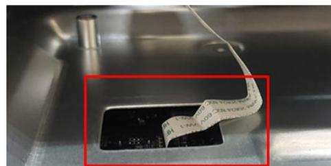
**S6** Unlock 3 screws to disassemble
